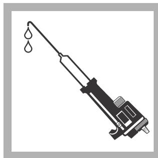
3. Hold the Digital Titrator vertically with the cartridge tip up. Turn the delivery knob to eject air and a few drops of titrant. Reset the counter to zero and clean the tip.
