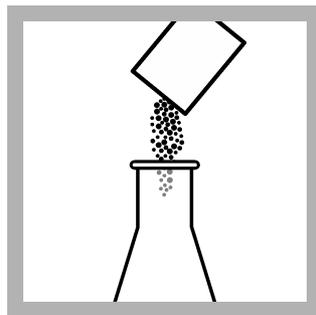
11. Add the contents of one Bromcresol Green-Methyl Red Indicator Powder Pillow. The indicator is not necessary if a pH meter is used.
