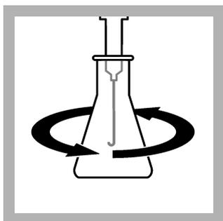
13. Put the delivery tube point fully into the solution and swirl the flask. Turn the knob on the Digital Titrator to add titrant to the solution. Continue to swirl the flask and add titrant until the color changes to a light pink color, or the pH is 4.5 (refer to [Table 2](#) on page 4 for additional pH endpoints). Record the number of digits on the counter.
