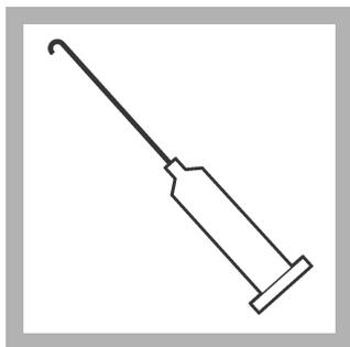
2. Insert a clean delivery tube into the 1.600 N Sulfuric Acid Titration Cartridge. Attach the cartridge to the Digital Titrator.
