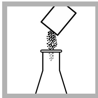
7. Add the contents of one Phenolphthalein Indicator Powder Pillow. The indicator is not necessary if a pH meter is used. If the solution is colorless or the pH is less than 8.3, the Phenolphthalein alkalinity is zero. Go to step [11](#).
