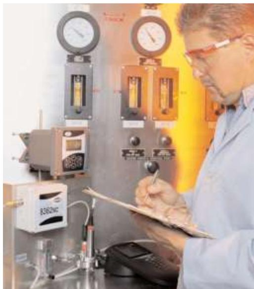
Dooley also noted that drift has been minimal during the several months the system has been in place, and that the design of the new flow cell makes it easy for his laboratory technicians to access the electrode and immerse it in buffer solution when calibration is required. Instrument set-up and calibration proved easy—even intuitive—simply by following the display menu.
