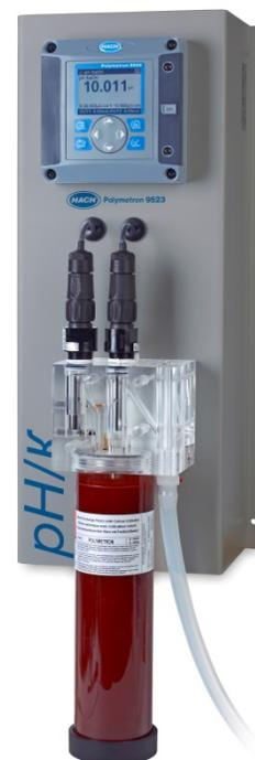
The conductivity  $k_{\text{spec}}$ , before the cation exchanger, is composed of the contribution from the sodium hydroxide (NaOH) and from the sodium chloride (NaCl) that is  $1/3 k_{\text{acid}}$ .
