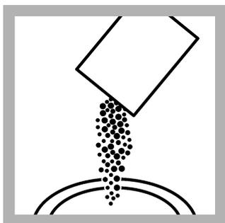
5. Add the contents of one BOD Nutrient Buffer Pillow to each bottle for optimal bacteria growth.
