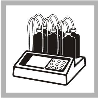
**9.** Put the bottles on the base of the BODTrak apparatus. Connect the tubes to the bottles and tighten the caps. Each tube is identified with the channel number. The channel numbers will show on the BODTrak display.
