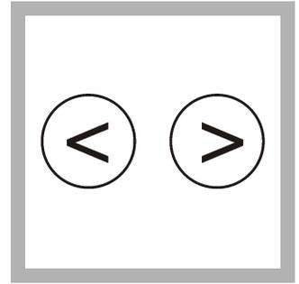
**12.** Push and hold the left and right arrow keys at the same time until the time menu shows. Push the CHANNEL 6 key to show the test length. Use the arrow keys to choose a 5-, 7-, or 10-day test (test duration is shown on the last line of the display). Push **OFF** to save selections and exit the menu.
