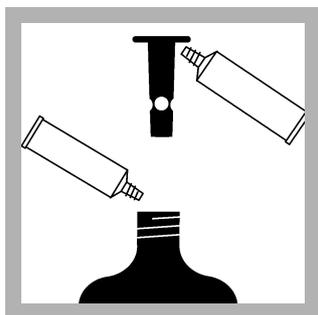
6. Apply stopcock grease to the seal lip of each bottle and to the top of each seal cup.
