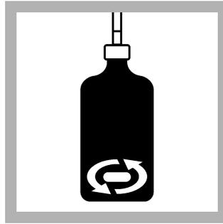
**11.** Make sure that all of the stir bars are in the center of the bottle and are rotating correctly. If a stir bar is on the side of the bottle, lift the bottle from the unit and carefully move it back. Do not start the channel test until the stir bar is rotating correctly.
