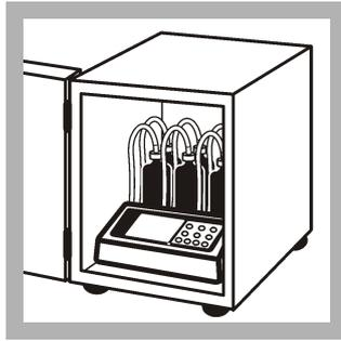
**10.** Put the instrument into the incubator. Set the instrument to on.
