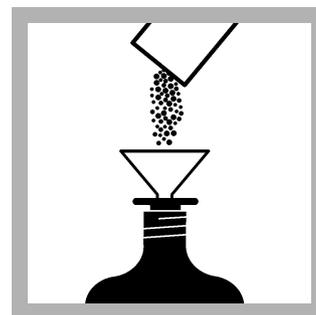
8. Use a funnel to add the contents of one Lithium Hydroxide Powder Pillow to each seal cup.
