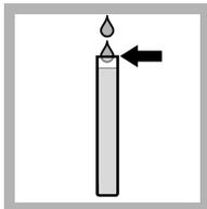
1. Fill the measuring tube with sample.
